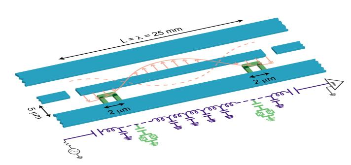
superconducting qubits inside a transmission line
