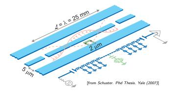
microwave pulses  $\Rightarrow$  lump element description inaccurate
